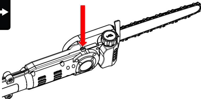
**UTILISEZ DE LA GRAISSE ET DE L'HUILE AU LITHIUM DE HAUTE QUALITÉ POUR ASSURER LA DURABILITÉ ET LA FIABILITÉ DE L'OUTIL.**
