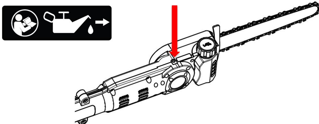
**USE HIGH QUALITY LITHIUM GREASE AND OIL TO ENSURE TOOL DURABILITY AND RELIABILITY.**
