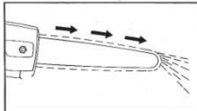
If there are not traces of oil, check to have refilled the tank.
